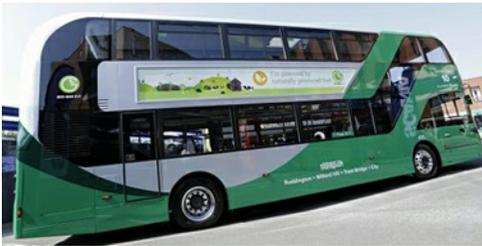
Moreover, the bio-gas buses are British built. The Scania chassis for each bus was assembled in Leyland in Lancashire, ahead of the bodying by Alexander Dennis in Scotland – and the Nottingham-based company Roadgas in Colwick has installed the fuelling facilities. These will also be available for use by other businesses.
